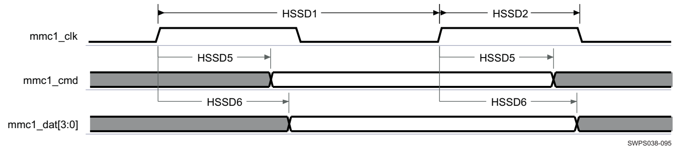
Figure 6-66. MMC1 Interface—High-Speed SD Mode—Data/Command Transmit
